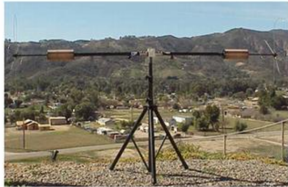
Center-fed pair of electrically short resonant whips (Hustler, etc.)
